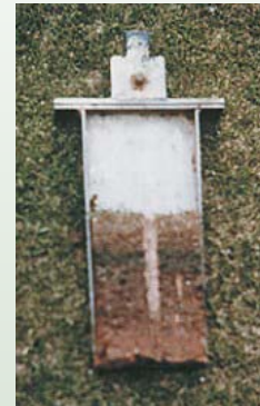
Many so-called 'aeration machines' only enhance surface drainage by creating a hole. They do little to increase the number or frequency of macropores.
