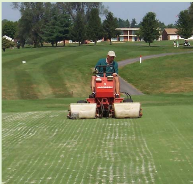
Following the DryJect procedure, we “dragged” the greens with Turf Groomer brush reels.
